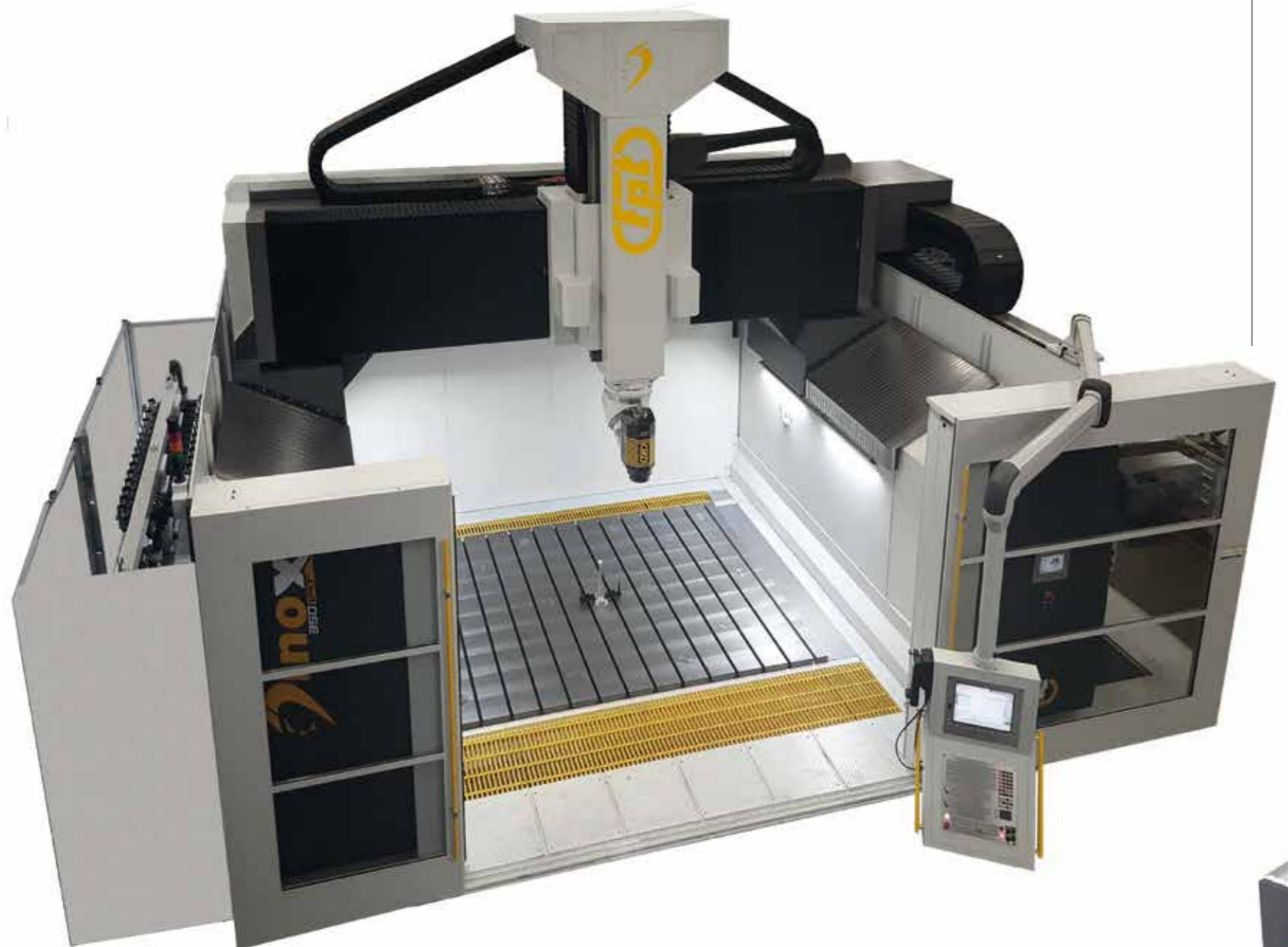
**DINOX 350** is a moving bridge Gantry-style machine suitable for heavy duty machining as well as high-speed cutting. The optimization of the structures, through use of the most advanced FEM analysis, and the use of drive systems of the most recent generation as well as linear motors, combine the need for high productivity with flexibility and accuracy, setting a new standard in the machine tool field.
