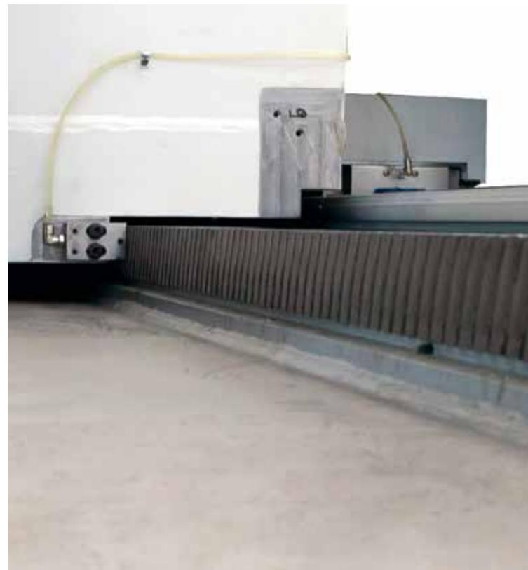
Dinox 350 equipped with DD (dual-drive) on the longitudinal axis and cross axis
