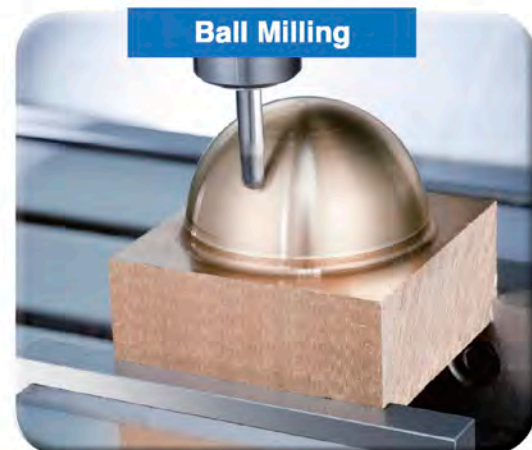
3D cutting test - circular ball milling
