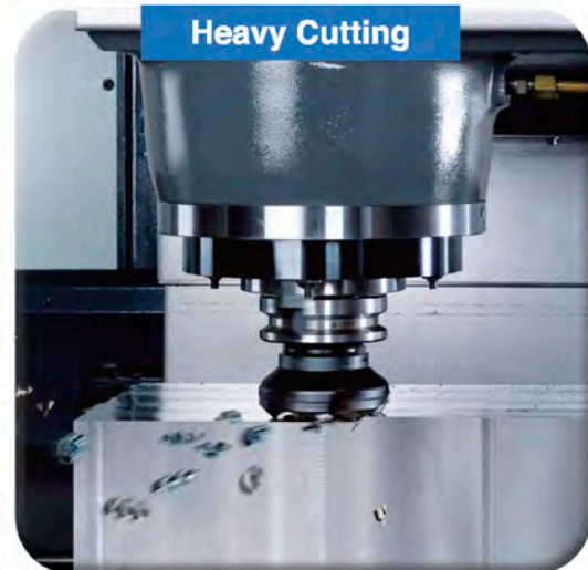
Heavy cutting test-face milling
