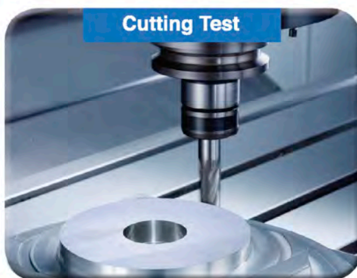
Light cutting test - 45° parallel and 2D circular milling
