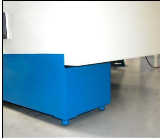
Figure 3-17: Place Sheet Metal Coolant Tank Slightly in Front of Machine Sheet Metal
