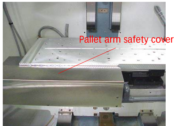
Figure 12-3 Remove Pallet Arm Safety Cover
