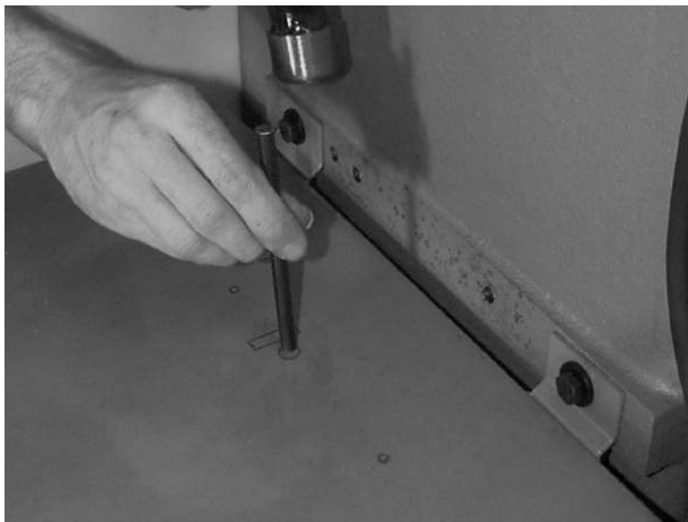
Figure 11-92 Center Punch Hole Locations for Drilling
