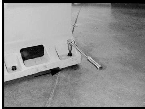
Figure 3-19 Drive Down Corner Leveling Screws
