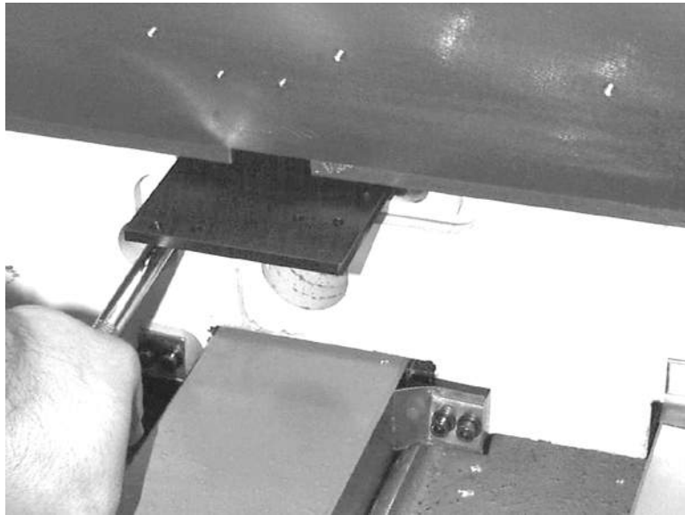
Figure 11-17 Install X Axis Scale Reader Mounting Screws
