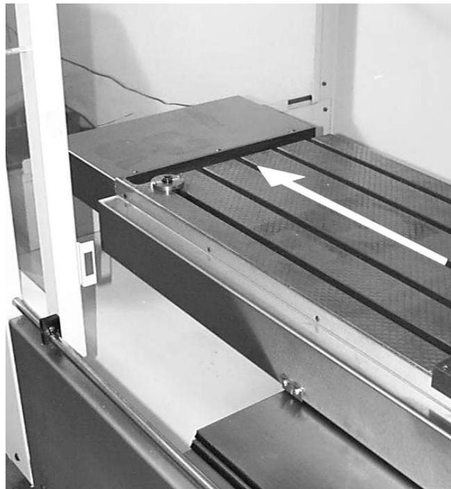
Figure 11-2 Jog Table to Maximum Negative X Axis Travel
