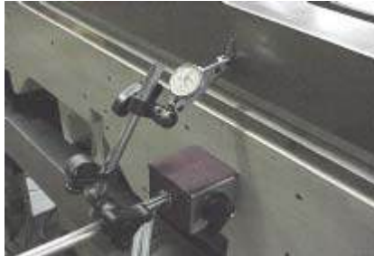
Figure 6-12 Set Zero Reading
