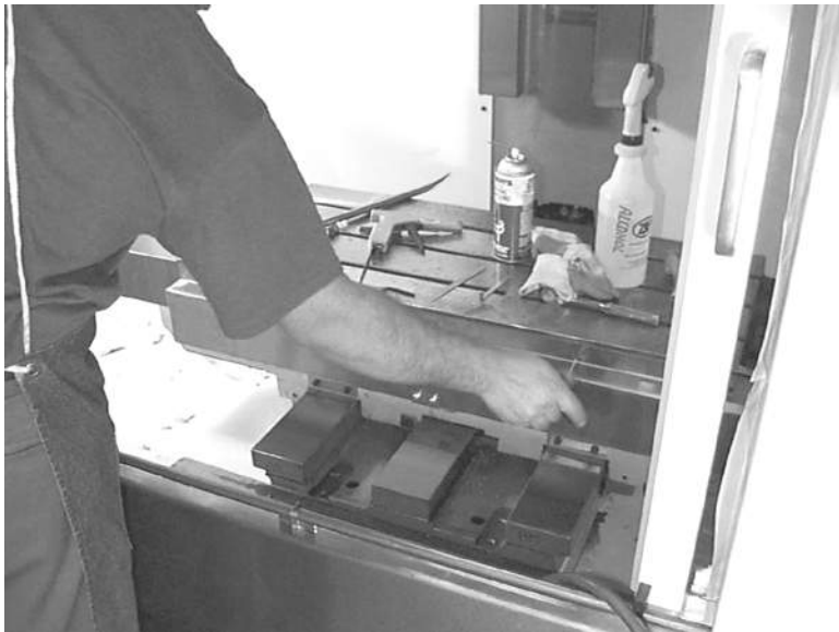
Figure 11-30 Attach Axis Position Indicator to Scale Cover
