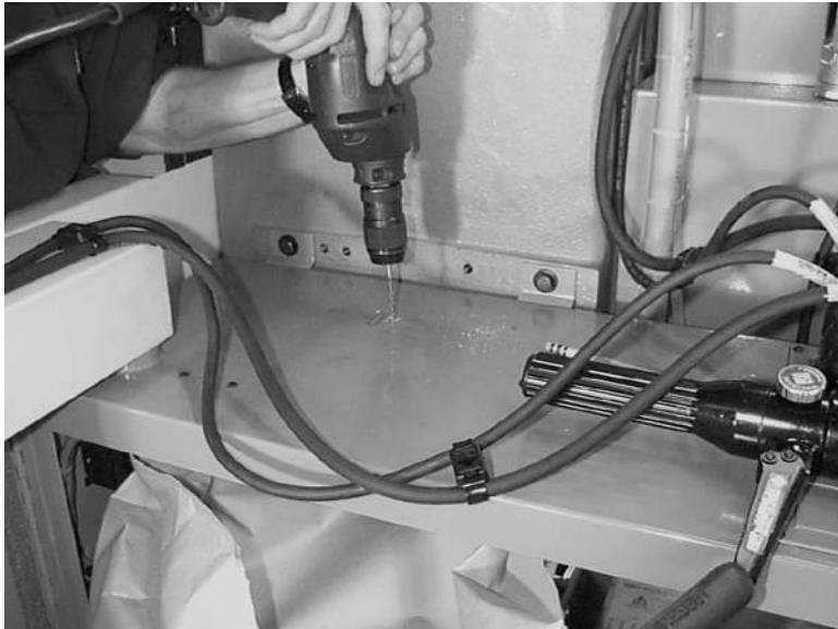
Figure 11-93 Drill Starting Holes
