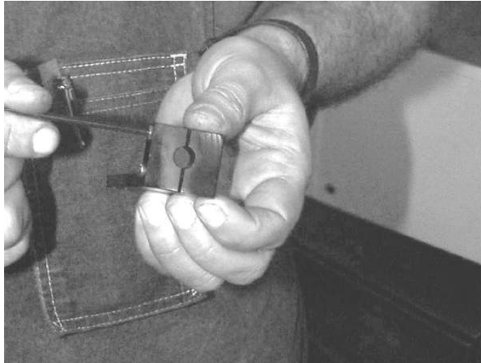
Figure 11-43 Insert Screw into Throw Rod's Saddle Mounting Bracket
