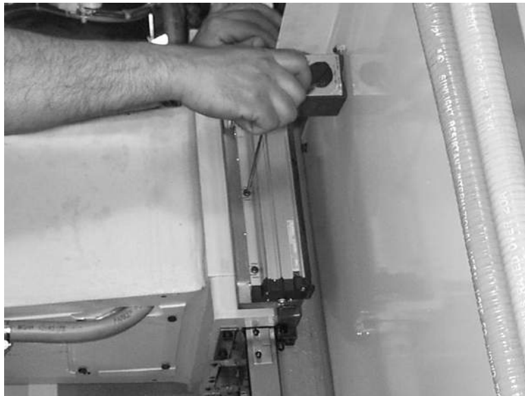
Figure 11-68 Attach Scale to Mounting Plate
