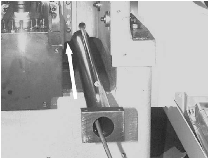
Figure 11-32 Insert Tube Through Column
