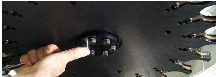
Figure 5-6 Loosen Hex Bolts Holding Tool Carrier
