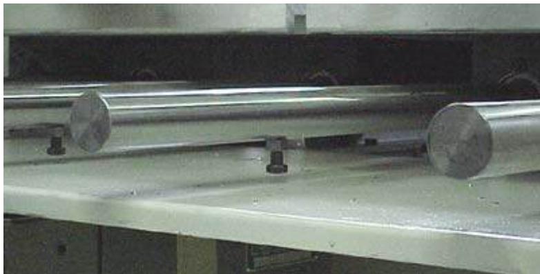
Figure 12-1 Verify Rail Support Bolts are Installed and All the Way Up
