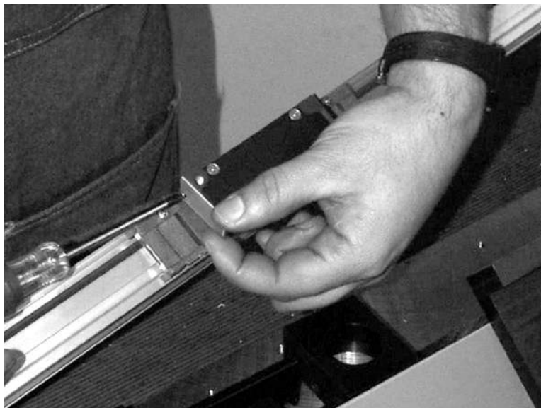
Figure 11-19 Remove Protective Cover from Pin Connector
