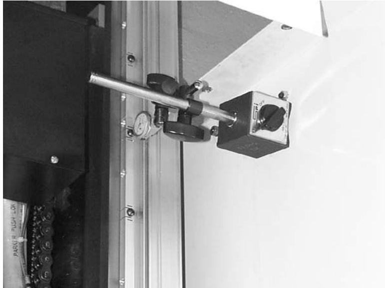
Figure 11-69 Set Dial Indicator Tip on Scale's Widest Ridge; Adjust Scale
