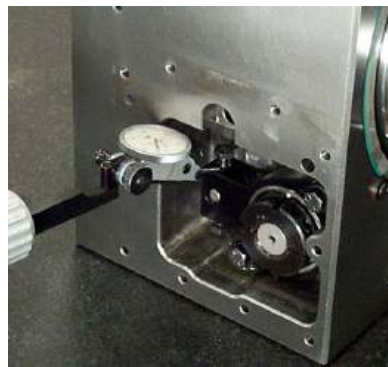
Figure 10-7 Zero Indicator on Worm Pivot Plate
