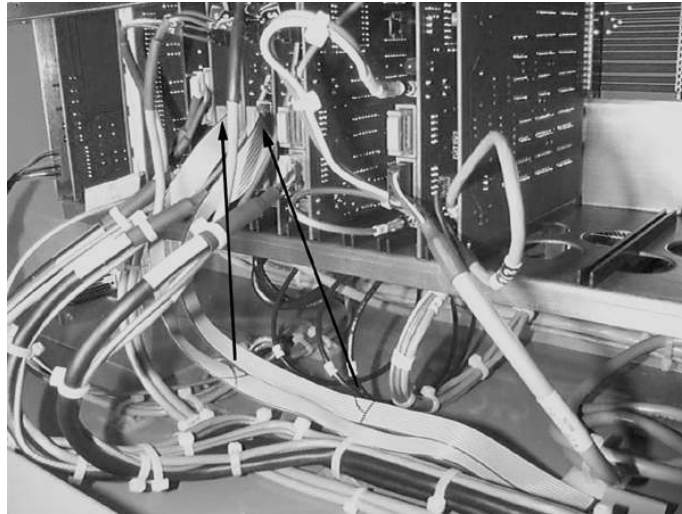
Figure 11-87 Secure Cable to Bottom of Cabinet
