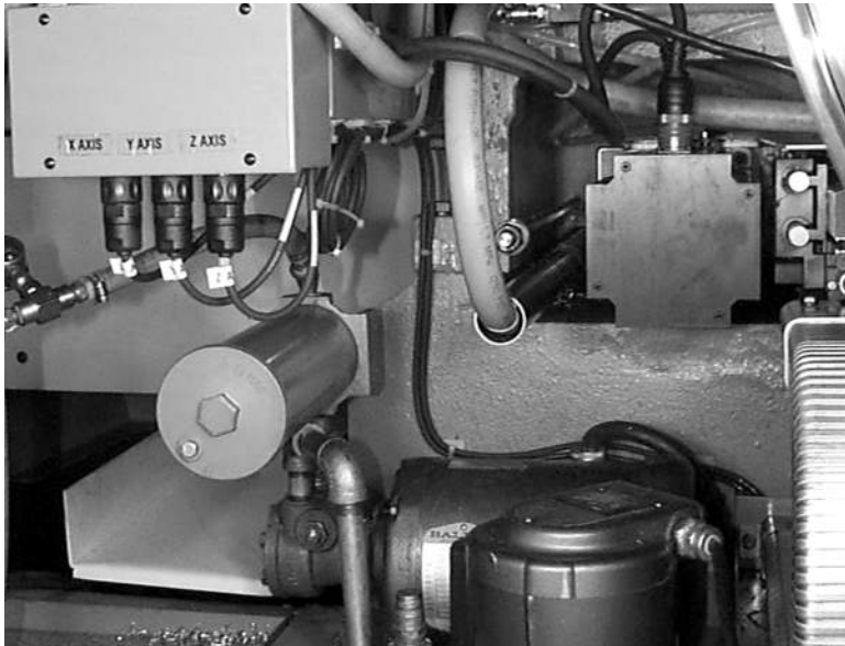
Figure 11-57 Route Cables to Back of Control Cabinet
