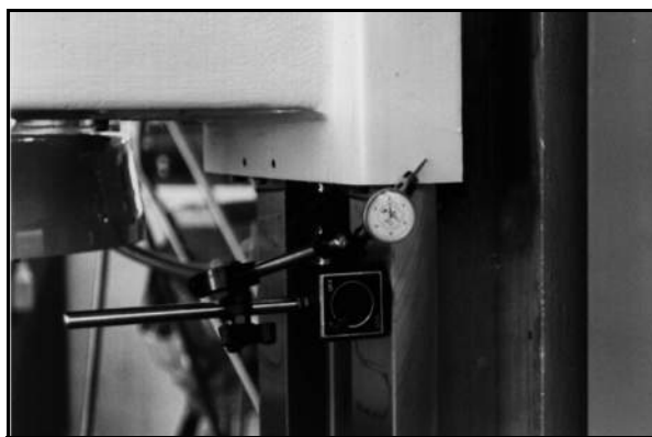
Figure 6-9 Magnetic Base and Indicator Mounting on Spindle Head
