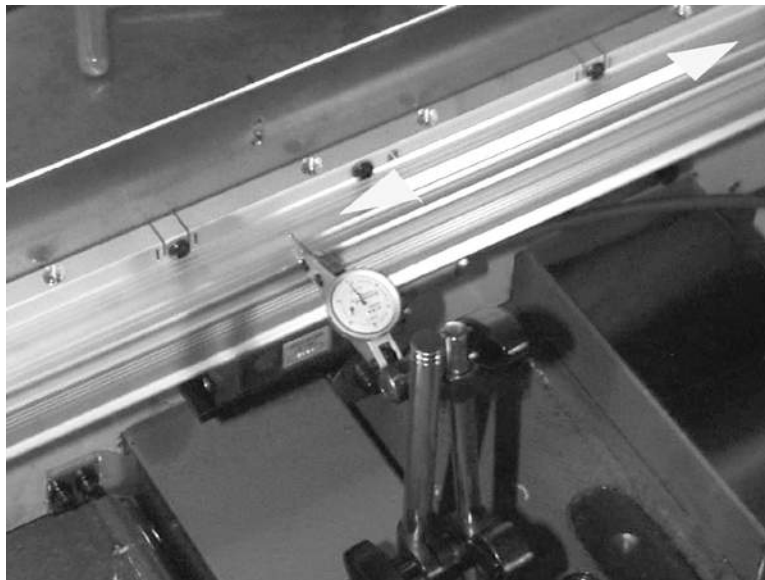
Figure 11-24 Mount Scale to Table
