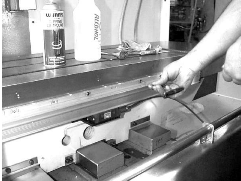
Figure 11-21 Attach Scale Assembly to Table
