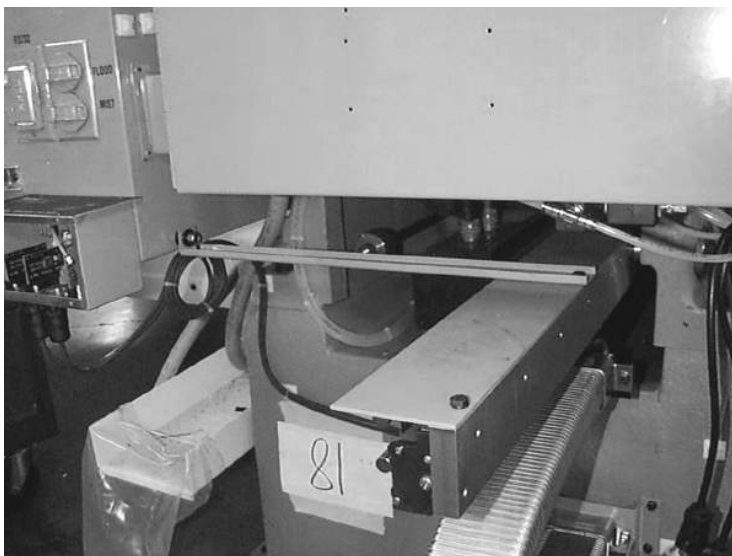
Figure 11-58 Attach Support Bracket Between Y Scale and CNC Junction Box (6030/8030)
