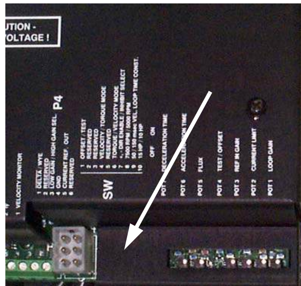
Figure 7-6 Switches are Preset
