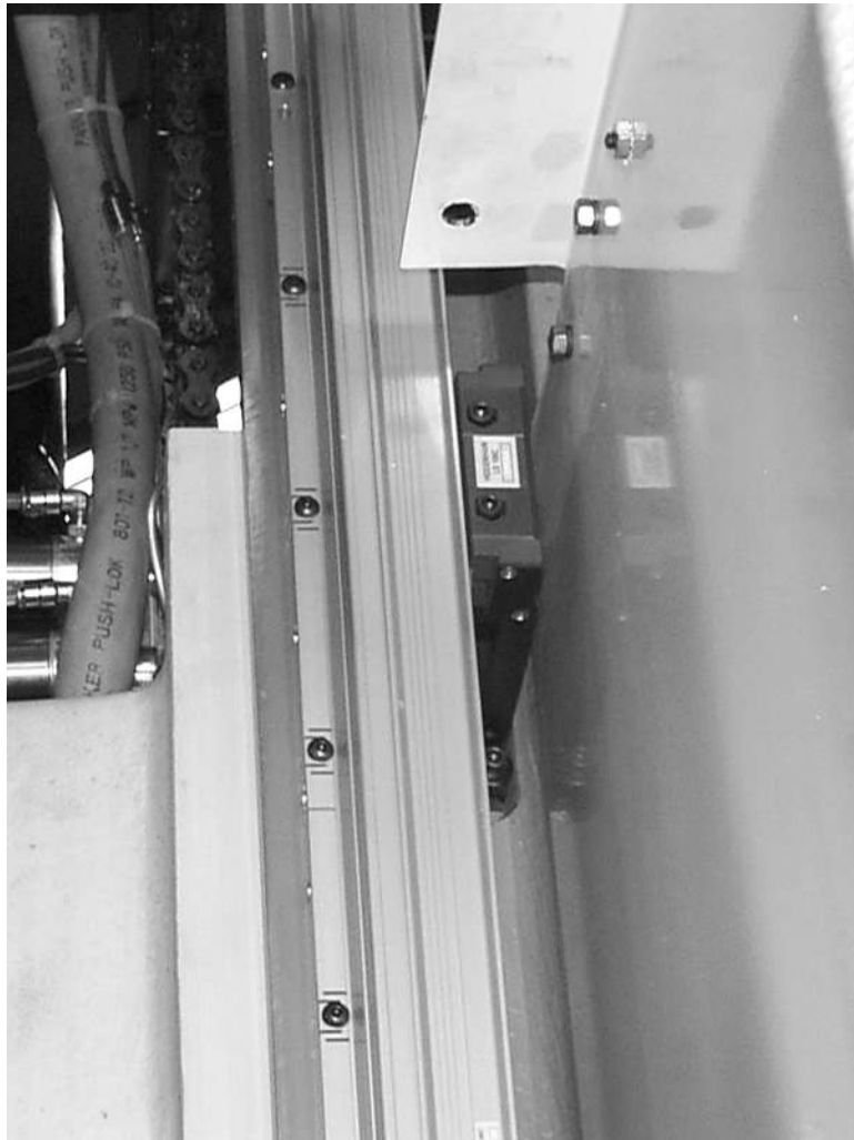
Figure 11-71 Attach Scale Reader to Mounting Bracket
