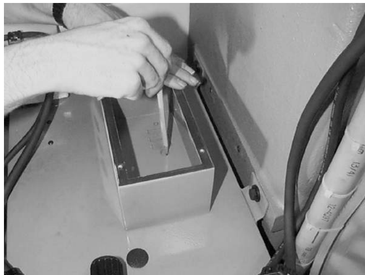
Figure 11-90 Mark Positions to be Drilled Out
