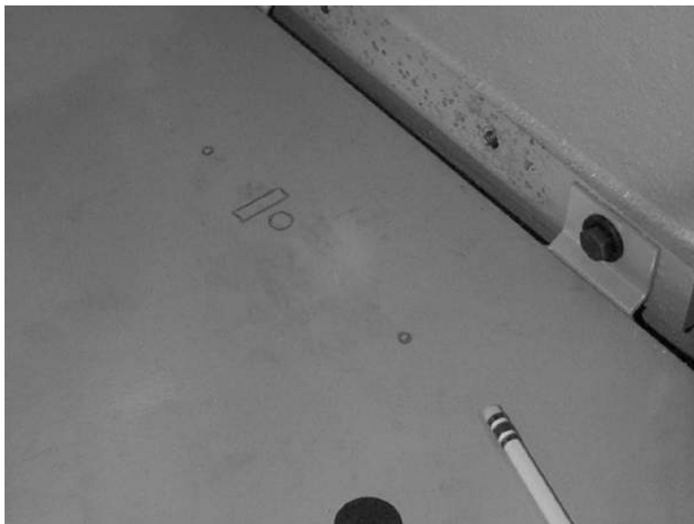
Figure 11-91 Mount Box on Top of CNC Cabinet
