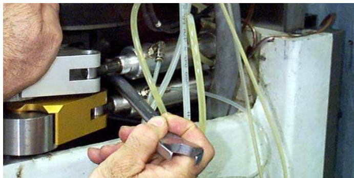
Figure 7-18 Remove Spindle Motor Bolt
