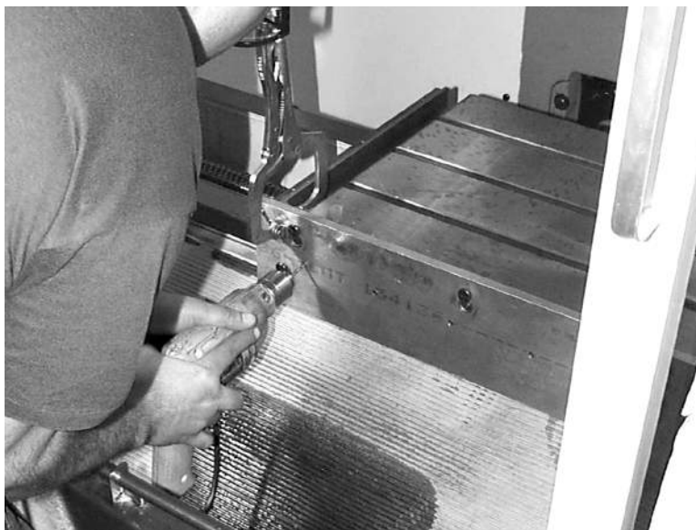
Figure 11-7 Drill Starting Holes
