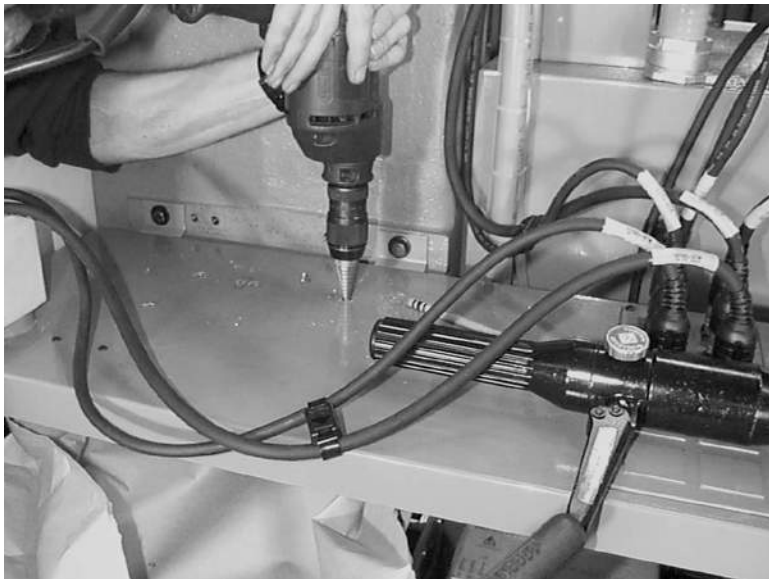
Figure 11-94 Open Holes with Step Drill
