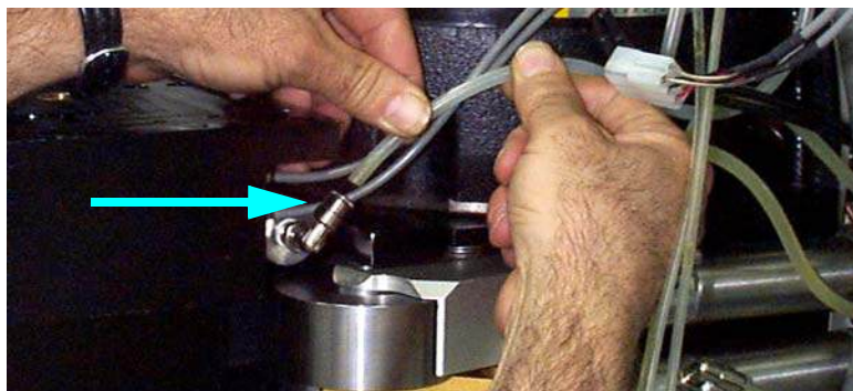
Figure 7-14 Disconnect Air Line to Orientation Piston
