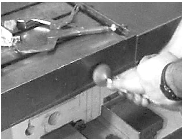
Figure 11-11 Clean Debris from Holes
