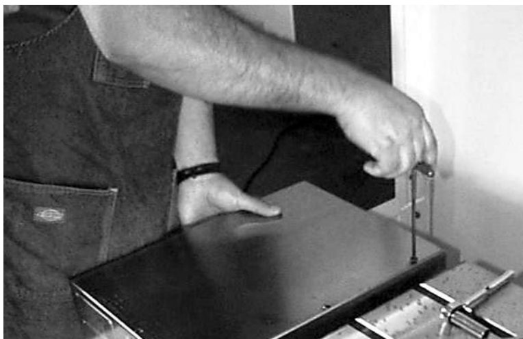
Figure 11-3 Remove Telescoping Way Cover
