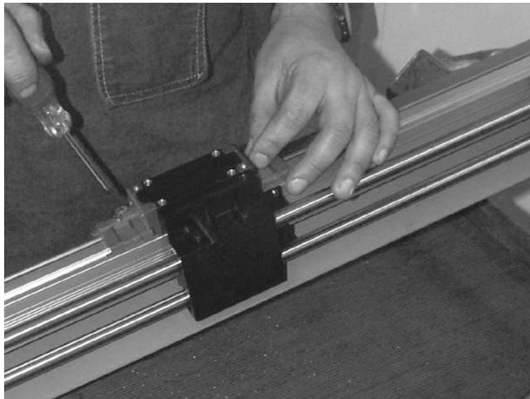
Figure 11-38 Remove Packing Clips from Scale Assembly
