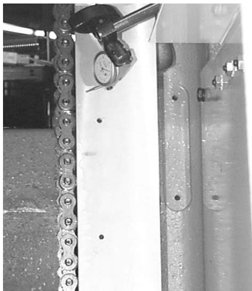
Figure 11-61 Mount Dial Indicator to Column
