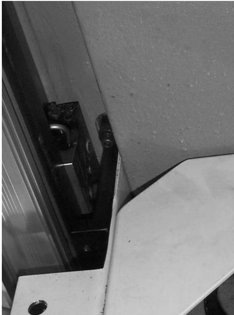
Figure 11-70 Attach Z Axis Mounting Bracket to Column
