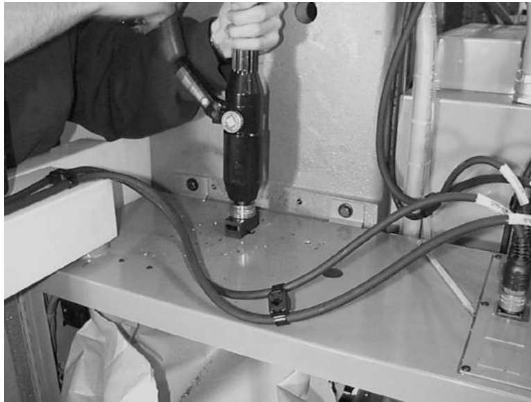
Figure 11-95 Create Opening for Fourth Axis Ribbon Cable
