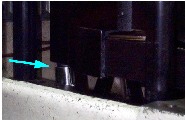
Figure 7-17 Remove Bolts to Rear Belt Guide
