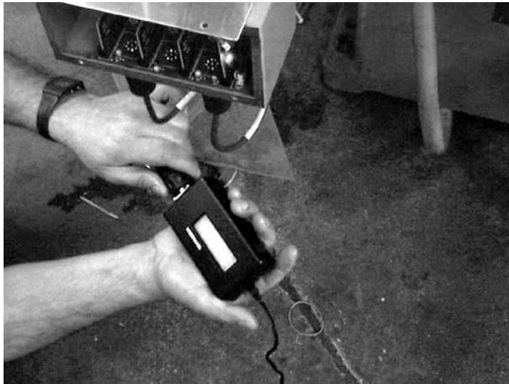
Figure 11-103 Plug Pin Connector Into Scale Test Box
